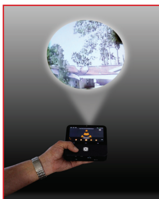
Streaming live via 4G through ZTE SPro2 hand held HD projector using VLC.
